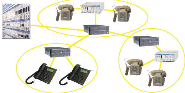
Figure 1. Asterisk can connect regular telephone lines and multiple VoIP standards.
