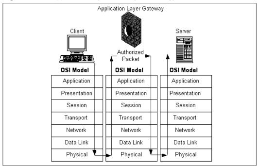
Figure 17.12 Application Layer Gateway Technology
