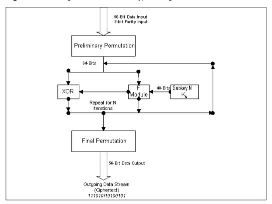
Figure 17.10 Diagram of the DES Encryption Algorithm
