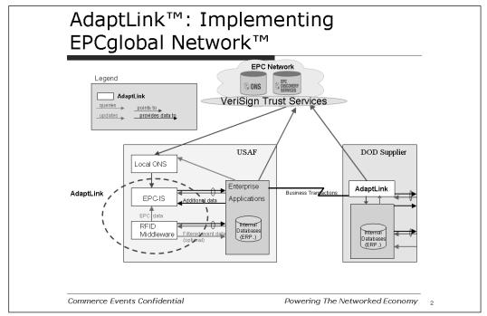
Figure 17.1 EPC Network Architecture—Components and Layers
