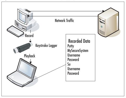
Figure 6.1 Sequence of Events for Keylogging Capture
