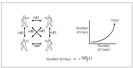
Figure 17.6 Symmetric Keys Required to Support Private Communications
