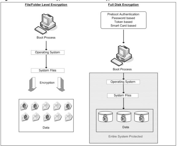
Figure 9.2 File Based Encryption vs. Full Disk Encryption
