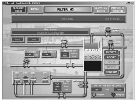
Figure 6.11 Iconics Plant Diagram and Control View
