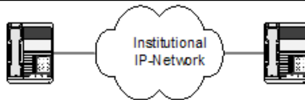
Figure 3.5: IP-Phone to IP-Phone without PBX
